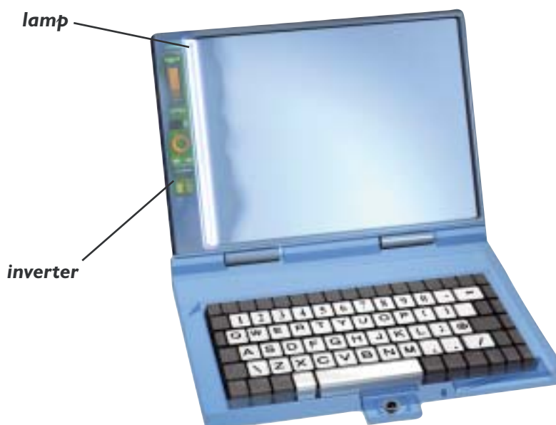
Fig.2 Example of Notebook computer with LCD backlighting
